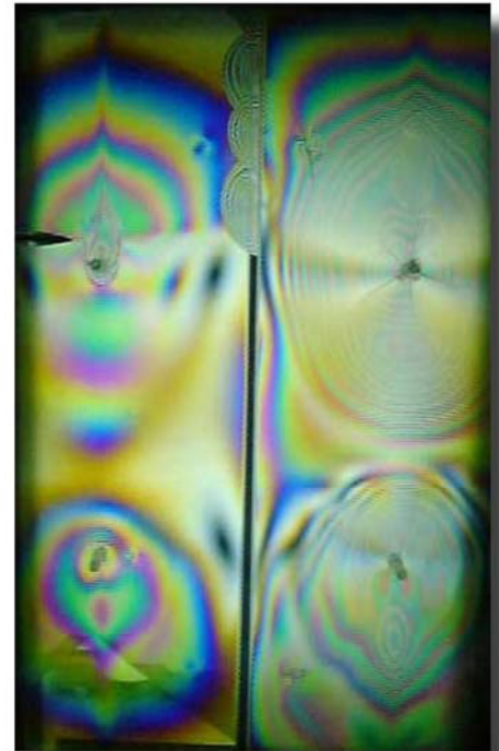
Figure 3: asymmetrical stress distribution for two sequentially injected parts. Upper gate was opened first. Left: packing pressure 20 bar; right, packing pressure 35 bar.
