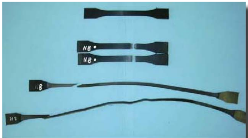
Figure 4: Tensile stress samples after test: brittle fracture for weld line area, ductile failure for other location. This second behavior was encountered for sequential injection specimens.
