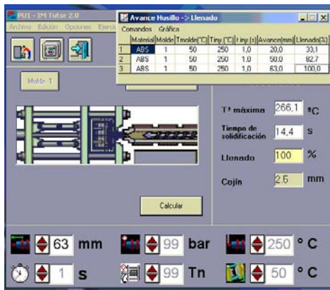
Figure 1: software developed to understand the setting up process
