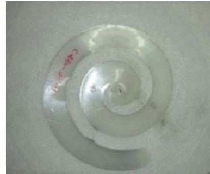
Figure 7: spiral mold used as basic tool to investigate textile over-molding.
